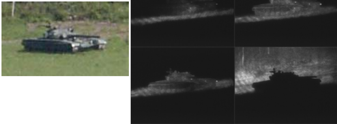
Figure 18. Left: A visual photograph of the scene used for gated viewing experiments. Right: Gated viewing images, captured using four different settings of the gate delay time. This results in the laser reflections from the front, entire, back, and background of the vehicle being imaged in the four frames. The range to the target is 0.9 km and the gate width 40 ns, corresponding to a physical depth of about 6 m.
