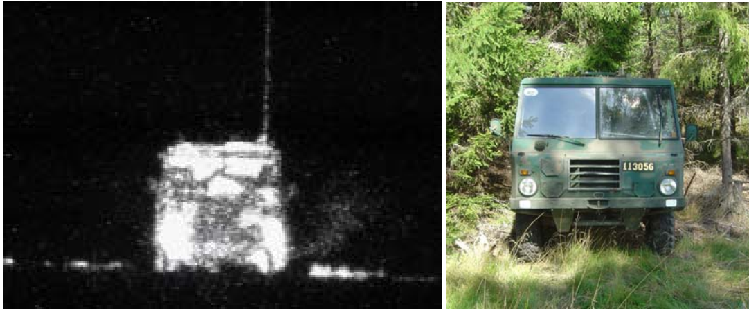
Figure 17. Image from a gated viewing system at night, showing two soldiers in the front seat of a command vehicle, both holding up their arms to cover a lamp. Notice the reflection in the headlights and the clearly visible antenna on the roof. For comparison, a similar vehicle is shown in the right photograph.
