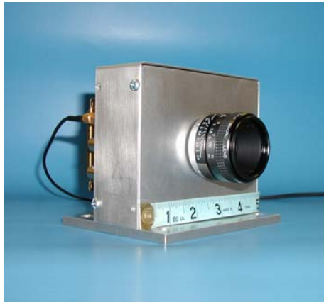
Figure 4. The flash 3-D sensor, excluding the illuminating laser. The scale is in inches. (Courtesy: R. Richmond, AFRL, USA)
