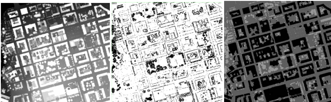
Figure 15. Left: Gridded height data ( DSM_{max} ). Middle: Multiple return image. Right: Classification results, buildings (black), vegetation (gray), roads (dark gray), posts (white).
