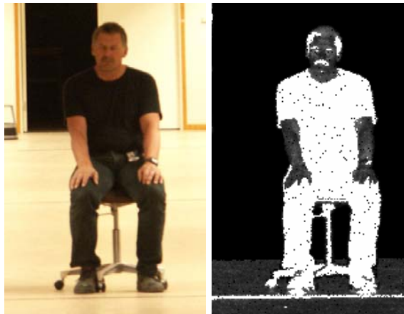
Figure 13. To the left a photograph and to the right a laser radar image (reflectance) at 1.5 \mu\text{m} wavelength. Note the high reflection from the clothes and hair compared with the reflection from the skin. Also note that the eyes were shut during the scan.
