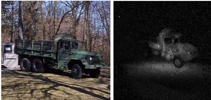
Figure 5. Example data from a flash 3-D laser radar (Courtesy: R. Richmond, AFRL, USA). Left: A photograph of a truck. Right: One range slice from a 3-D image. The image is slightly processed at FOI.
