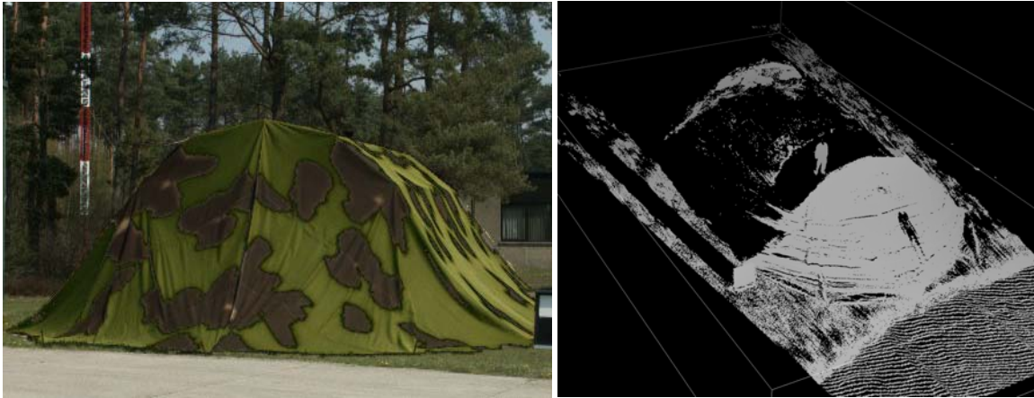
Figure 10. A photograph of a vehicle camouflage shelter to the left. To the right, a re-projected 3-D laser radar image (last echo) of the scene, also revealing a man standing in the middle of the shelter. Note the low reflection from the face. As the last echo is recorded, the pulse returns from the man under the net cause a “shadow” on the front of the net.
